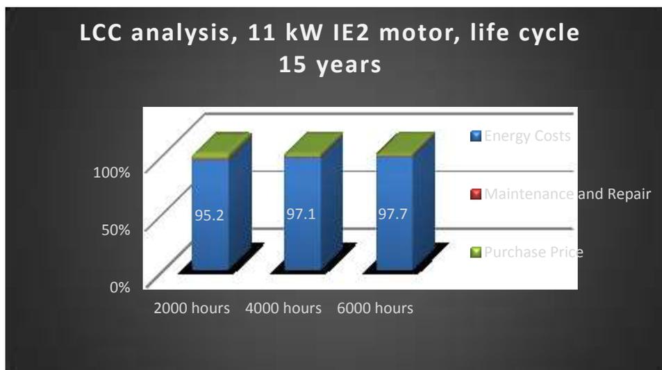
Figure 4 – LCC analysis, 11 kW IE2 motor, life cycle 15 years (Source: (Almeida, Ferreira, Fong, & Fonseca, 2008)
