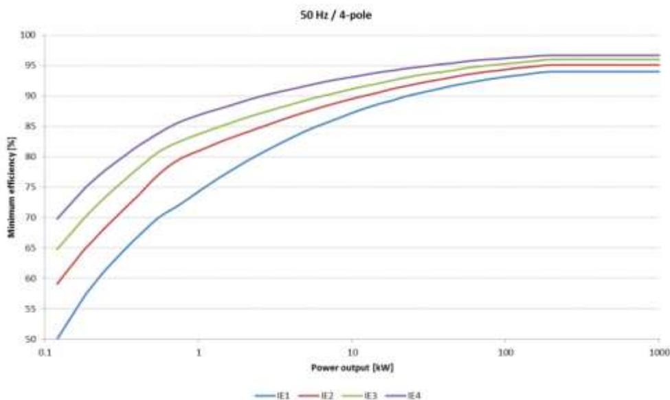
Figure 1 – IE class for 50 Hz 4-pole motors according to IEC 60034-30-1:2014
