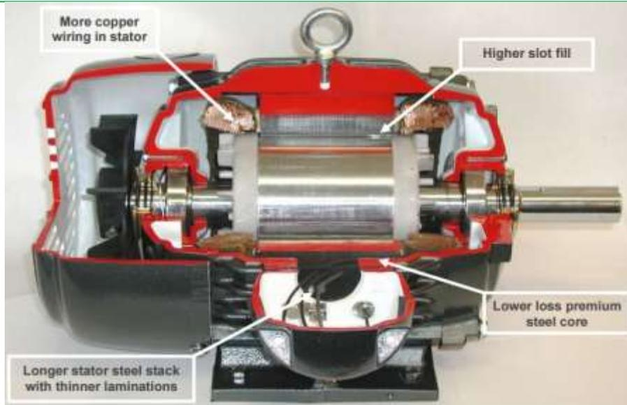
Figure 3 – Inside of a IE4 motor
